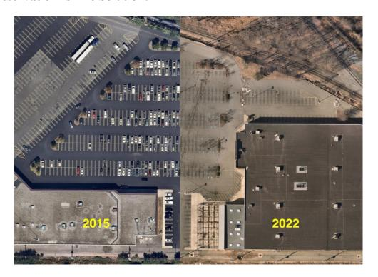
Asphalt begins to age immediately following installation. Private paving projects (Commercial or DOT asphalt mixes) have a higher percentage of recycled asphalt introduced into the mix designs which cause them to oxidized and become brittle sooner. The days of being able to install a parking lot and then wait 20-30 years till
